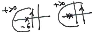
$$\underline{x}_1 = x(0) e^{st} \Big|_{s=-6} ; \quad \underline{x}_2 = \frac{1}{1!} \frac{d}{ds} e^{st} \Big|_{s=-6}$$
